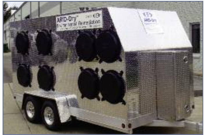
Advanced filtration system enclosed trailer - 18,000 SCFM
